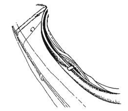
14 Attach folding keel section to bow and stern keel frame sections
