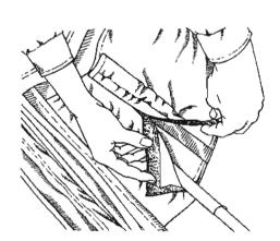
b) The seat sling bar has white plastic spacers. Push the stern end of the bar behind the large crosspiece. The seat sling bar rests on the gunwale bar. The plastic spacer faces into the kayak. Push bow end of sling bar behind aluminum plate.
