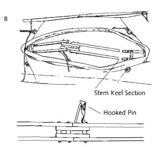
Push down keel section, and lock into place with long, hooked pin.
