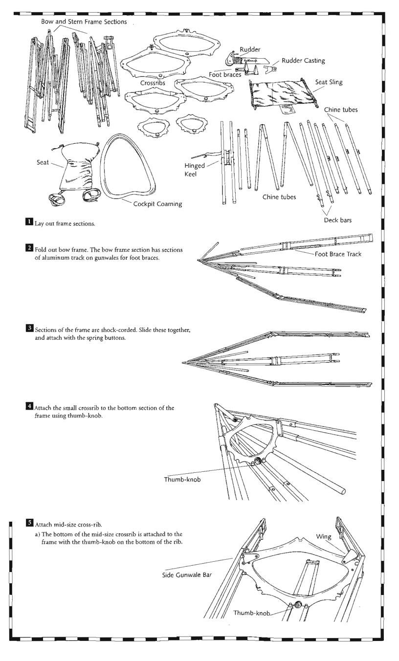
5 b) The sides of the rib slide into the bow gunwale bars. Close the side "wings" to fix into place.
